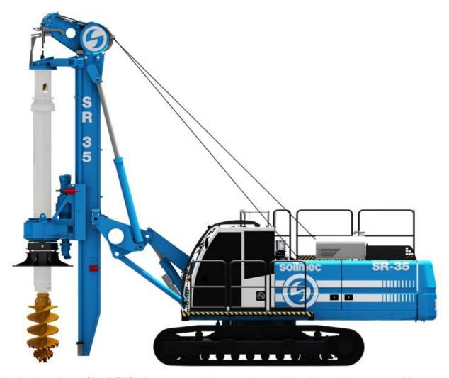
In the brand new <u>SR-35 EVO</u>, the segmental mast engineered for this unit is composed by two elements linked by a flange. Such a design allows to shorten or to extend the mast according to the job site needs without removing the section linked to parallelogram system. The solution enables to rapidly convert the rig machine in to the LHR configuration.
