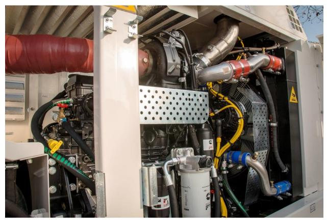
The brand new <u>SR-35 EVO</u> is installed with the latest generation Stage-V Diesel engines set up with the low idle control able to improve efficiency and mitigate noise pollution. The selected engine is the Cummins B6.7. It is an extremely powerful engine, it is efficient and flexible and finally helping the operator to easily deal with the most demanding jobs. Compared to the SR-30, this new engine allows 5% lower specific fuel consumption even by delivering up to 12% more power.
